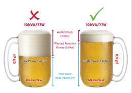
Real Power (Watts) = Apparent Power (VA) X Power Factor (PF)
